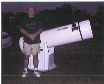
BIG DOB. Dobsonian-mounted reflectors have revolutionized astronomy by offering big apertures at low cost. MAGGIE MCKEE
