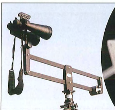
HOLD STEADY. Astronomical binoculars can be heavy, and using them is easier with a parallelogram mounting. MAGGIE MCKEE
