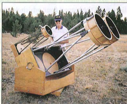
GETTING IN DEEP. Really dedicated skywatchers have setups far beyond what most beginners imagine. In certain cases, that means building 20-inch Dobsonian-mounted binoculars. MARTY CURRAN/MAGGIE MCKEE
