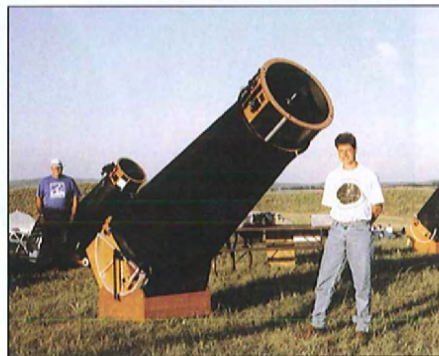
BIGGER DOB. Really big Dobs pull in lots of light. Fortunately for owners, they disassemble for transport. MARK DAHMKE
